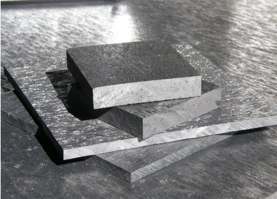
polyonyx+<sup>®</sup> is a stage flooring product made from aerated polymers that is inherently black, easy to cut with standard woodworking tools, available in four thicknesses, comes in 4x8 sheets and is incredibly durable. The product is an excellent replacement for 1/4" hardboard flooring typically found on stages. The following points should be followed when using the product as an overlay over an existing stage floor.
